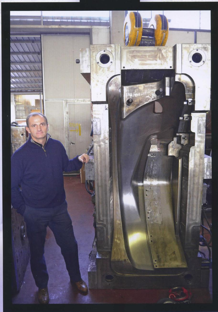
In its in-house technical department, equipped with sophisticated design and machining centres, experienced designers can develop dies according to customers' requirements, including the design and production of large injection tools.
